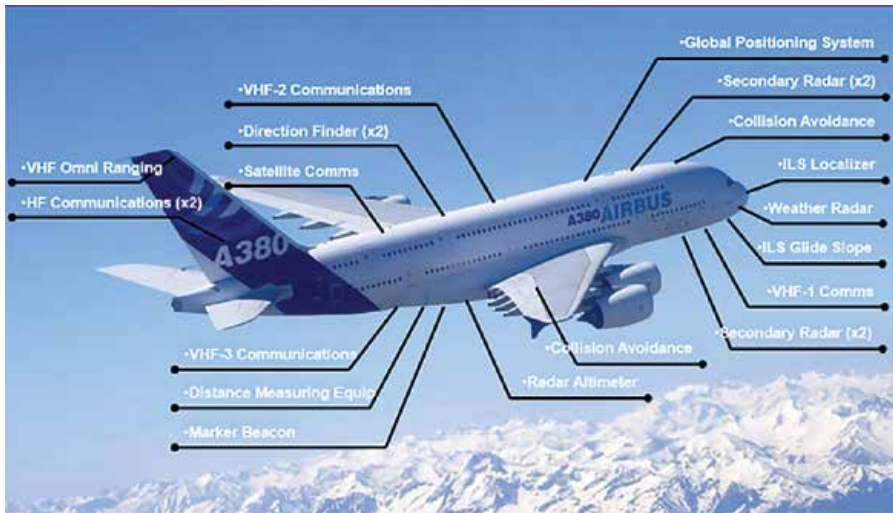
Figure 1.7. Airbus A-380 electronic systems. (Source: FAA.)
